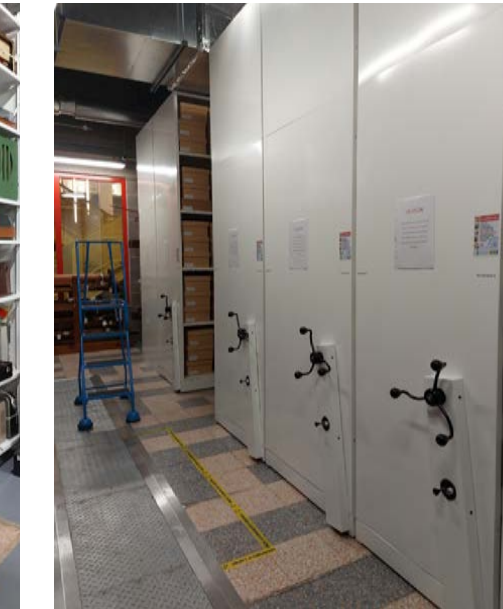
Example of rolling racking system (manually operated) at The Secret Collection, Paisley
